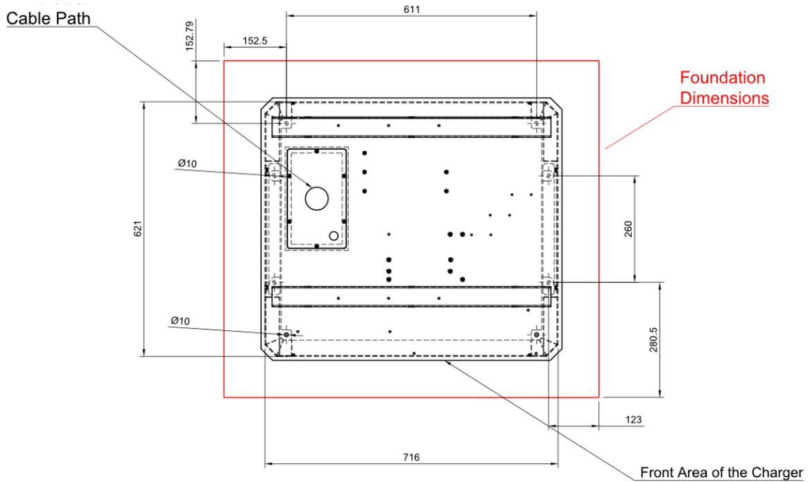
The below figure indicates the dimensions of the foundation for the BE-M Series CHARGING STATION.
