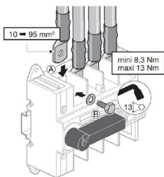
5. Connect the phase and neutral conductors in the following order:
