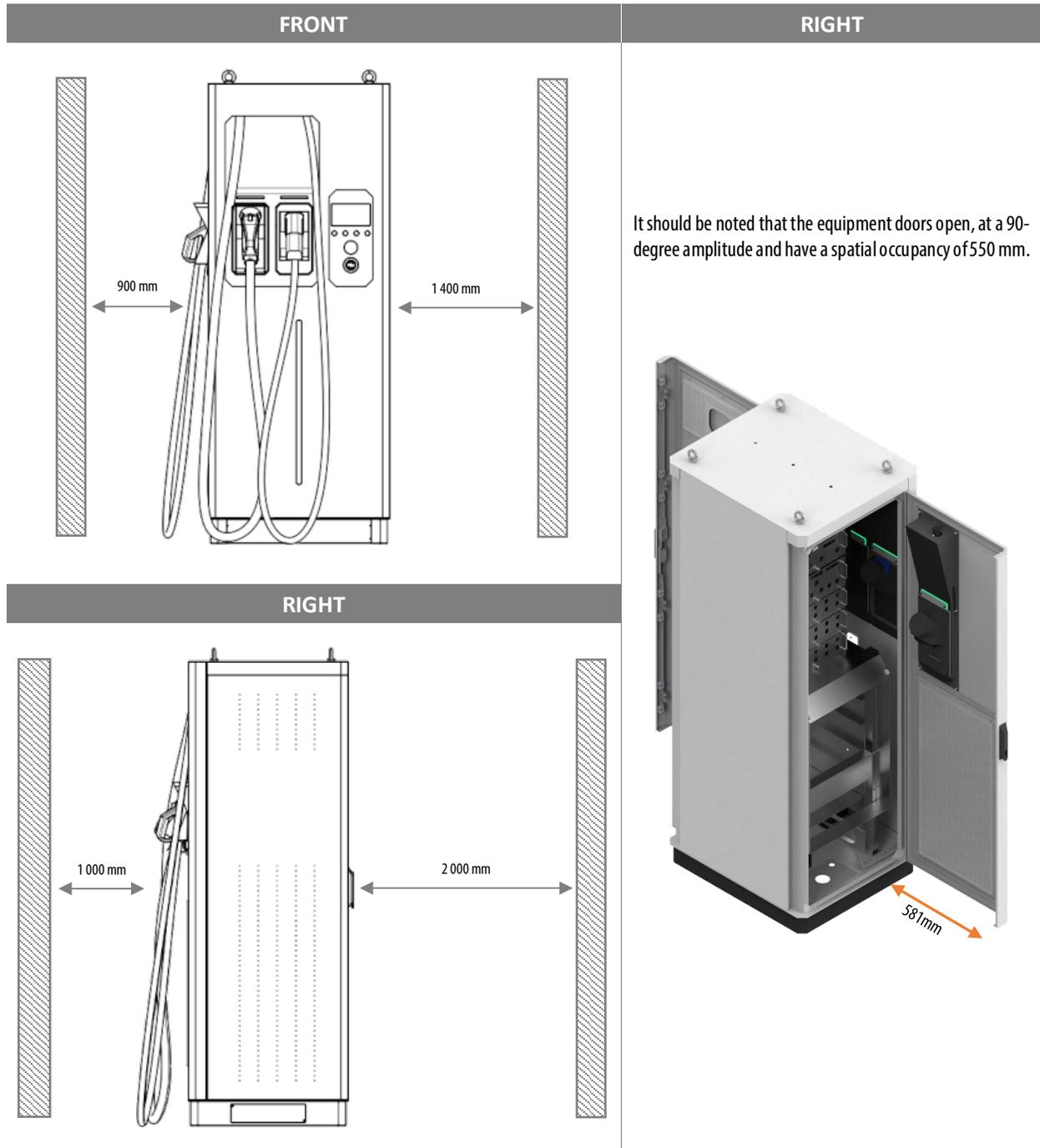
Fig. 3 - Minimum required space around the equipment
