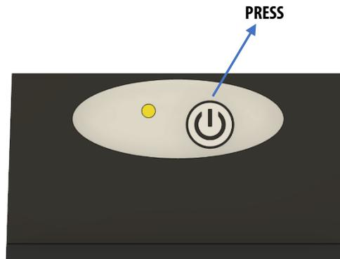
3. After pressing the ON button, if the equipment is still not connected to the mains, the signal RED by the UPS will appear due to mains fault.
