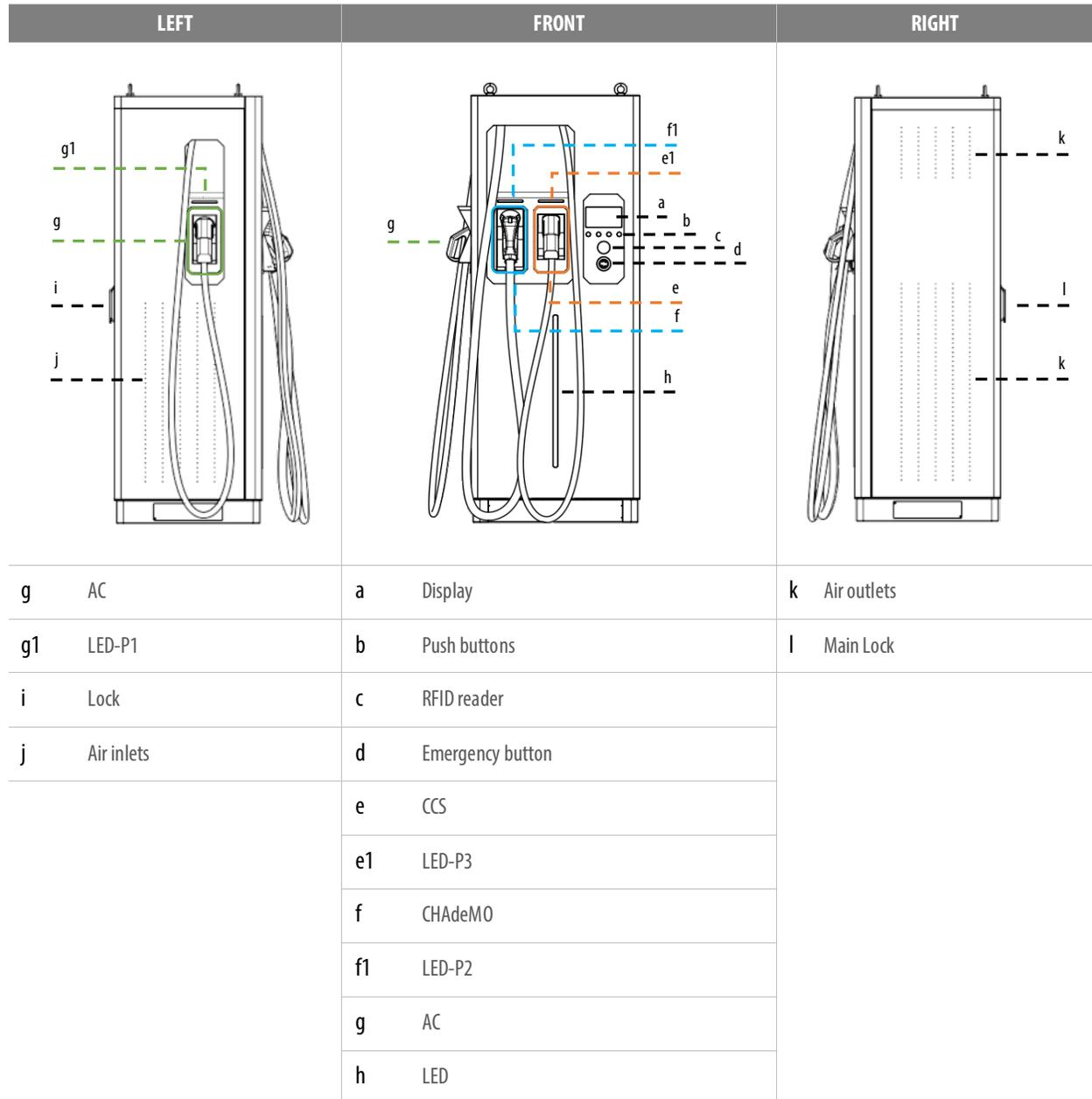
Fig. 1 - Description of the CHARGING STATION's elements
